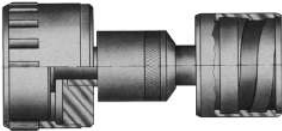
Basic design GZ roller burnishing tool
