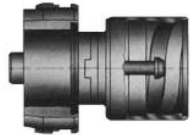
Basic design SK skiving head
